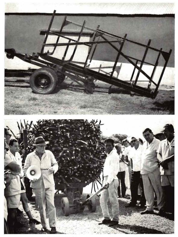
Top: Self-loading trailer (patent applied for). Bottom: Demonstration by inventor of a new hitching device for train of trailers (patent applied for)
