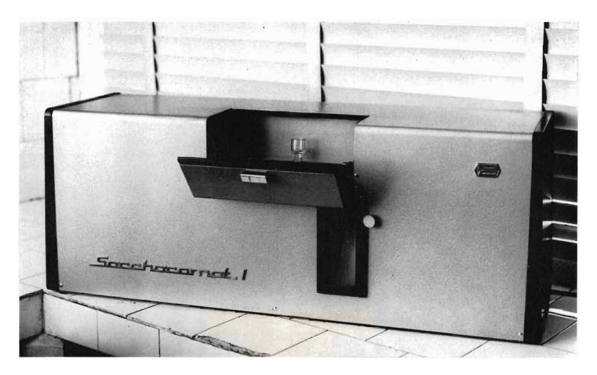
Automatic polarimeter used for the first time in a sugar factory (Union St. Aubin)
