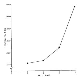
Fig. 10. Increase in dextran % Brix along milling tandem
