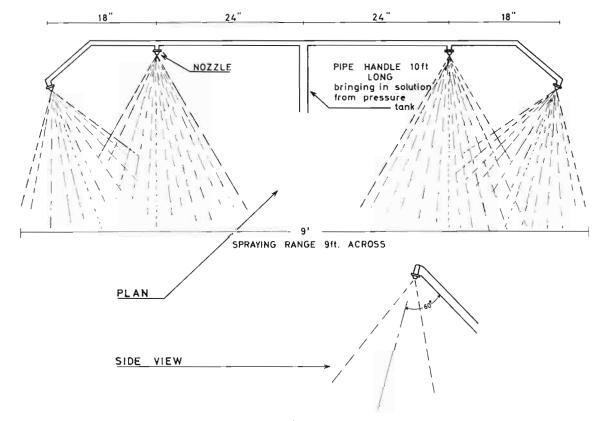
Fig. 28. Details of special boom designed for spraying with DA5.
