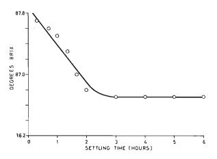
Fig. 32. Effect of settling time on spindle Brix of a 1: 1 wt/wt final molasses solution.
