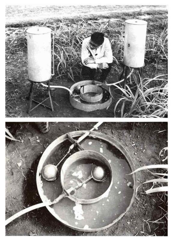
Determination of water infiltration rate by means of the cylinder infiltrometer
